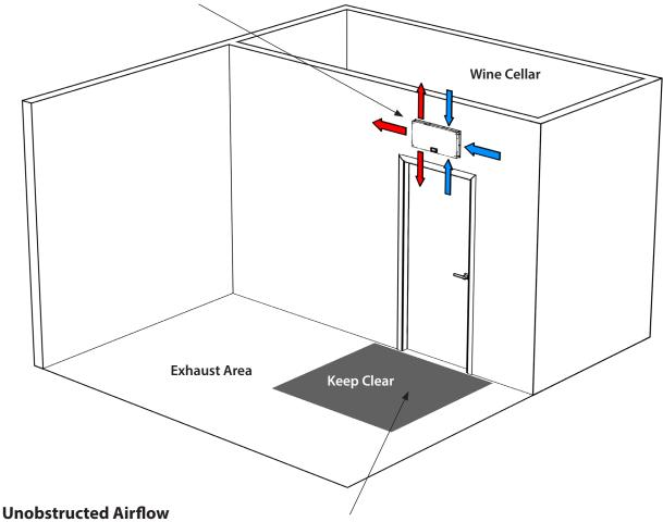
Unobstructed airflow to and from the unit is critical to the unit's overall performance and lifespan. Make sure there is a minimum of three (3) feet of horizontal clearance in every direction around the unit (five feet is ideal). The air blown by the fans needs to circulate and either dissipate or absorb heat from the space. The system will operate more efficiently with a greater amount of air to exchange.
