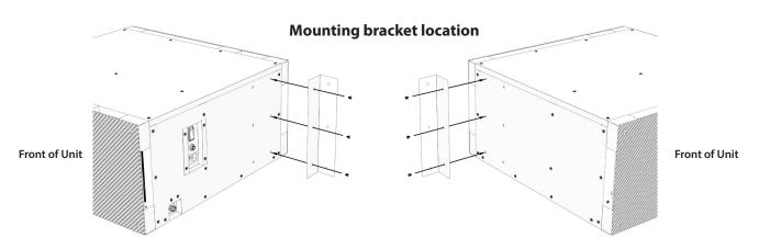
**STEP 4**Secure the two brackets to the corresponding side of the cooling unit on exterior side of the cellar. There are two mounting positions available.
