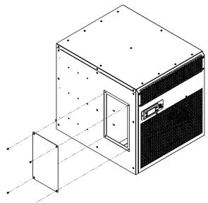
Remove the (4) screws and side access panel to view internal drip tray.
