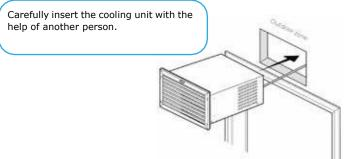
Note: Be careful not to damage the unit when setting it in place.
