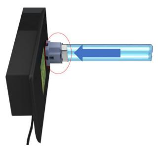
Install new bulb into the UV base. **\*NOTE: Do not touch the glass portion of the germicidal UV lamp with bare hands.** Use cotton gloves or rag to avoid skin oils that will harm the UV lamp.
