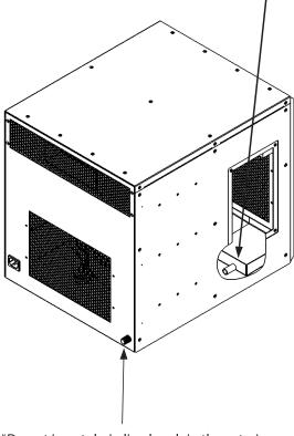
\*Do not insert drain line brush in the exterior drain port.
