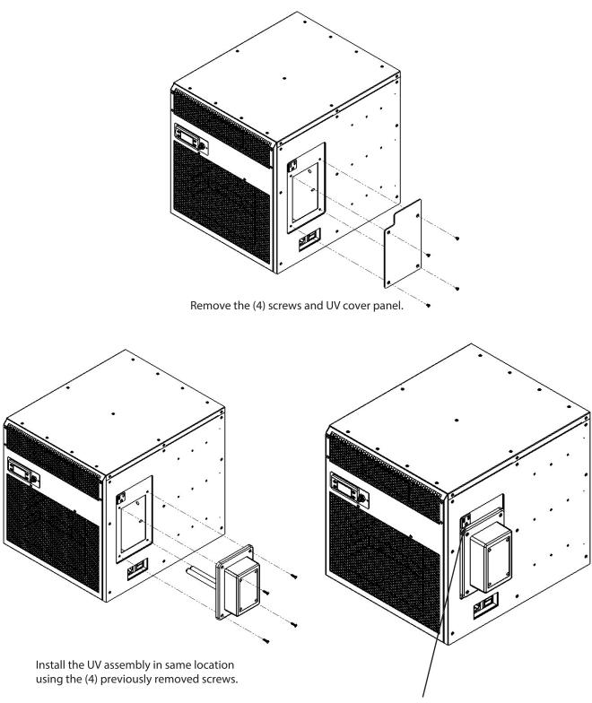
Plug the UV assembly power cord into the UV power receptacle
