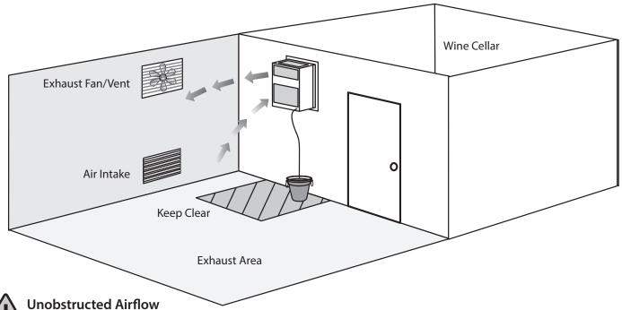
Unobstructed airflow to and from the unit is critical for the unit's overall performance and lifespan. Make sure there is a minimum of three (3) feet of horizontal clearance in every direction around the unit (five feet is ideal). The air blown by the fans needs to circulate and either dissipate or absorb heat from the space. The system will operate more efficiently with a greater amount of air to exchange.
