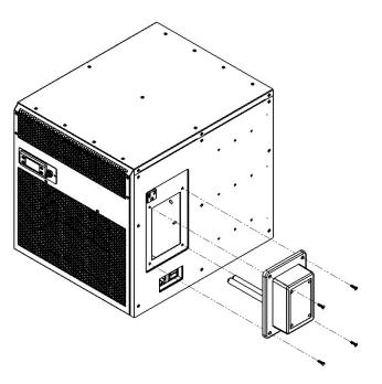
Install the (4) screws and UV assembly.
